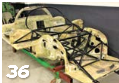
908 Chassis and underbody at Porsche Restoration Shop.
