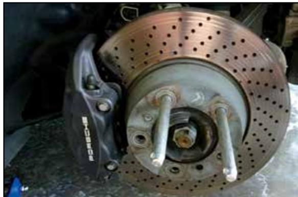
Two Gewindebolzen as on/off guides for the wheel/tire combination.
