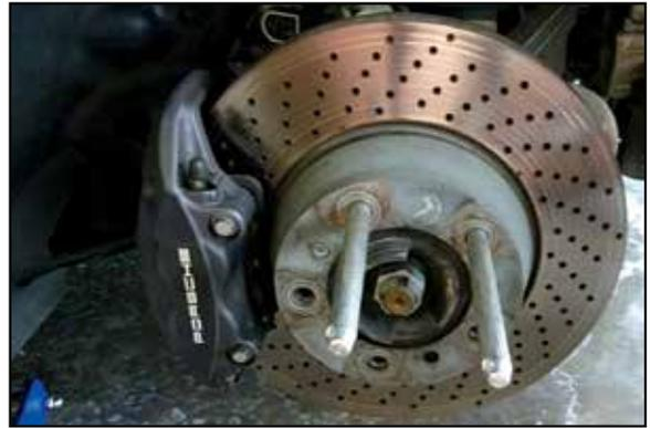
Two Gewindebolzens as on/off guides for the wheel/tire combination.
